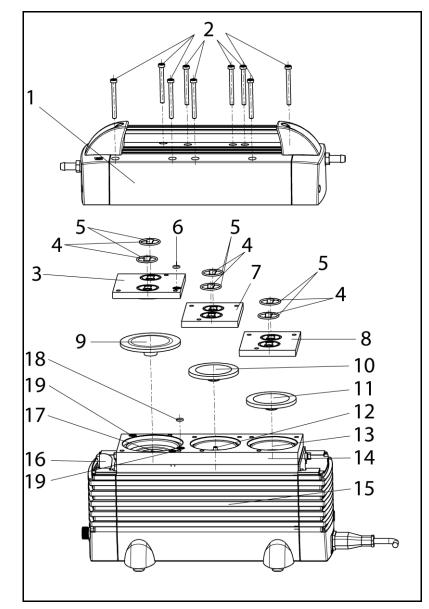
Fig. 6: Exploded drawing N 920 AP.18 / N 920 AP.29.18
