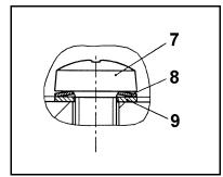
Fig. 10: Position and orientation of disk (8) and washer (9) at screw (7)
