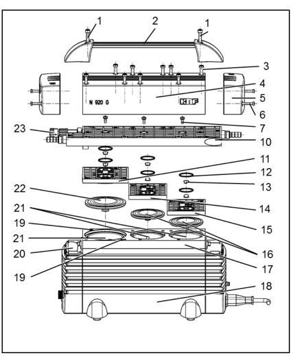
Fig. 8: Exploded drawing N 920 KT.29.18G
