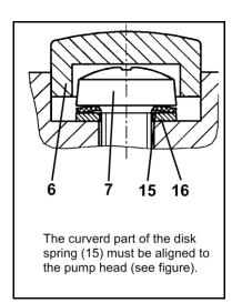
Fig. 14: Orientation disk spring
