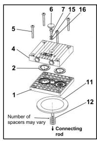
Fig. 13: Pump head (Exploded drawing)
