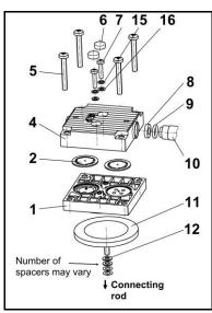
Fig. 10: Pump head (exploded drawing)
