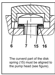
Fig. 11: Orientation disk spring
