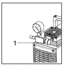
Fig. 8: Fine-adjustment valve
