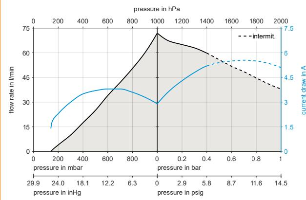
Flow rate determined at 20°C, 1000 hPa with air
