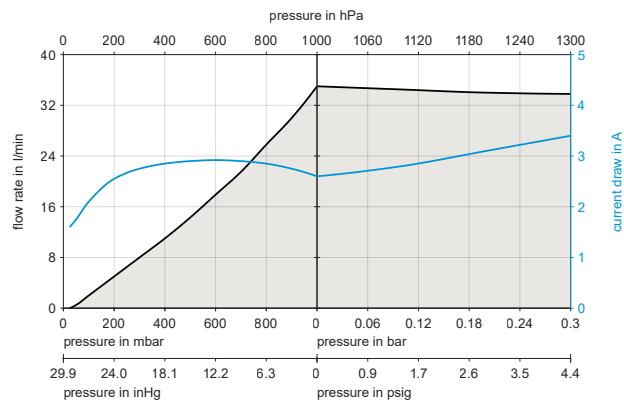
Flow rate determined at 20°C, 1000 hPa with air
