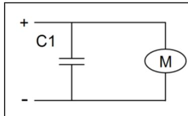
Fig. 3: Electrical diagram of the supplemental circuit
