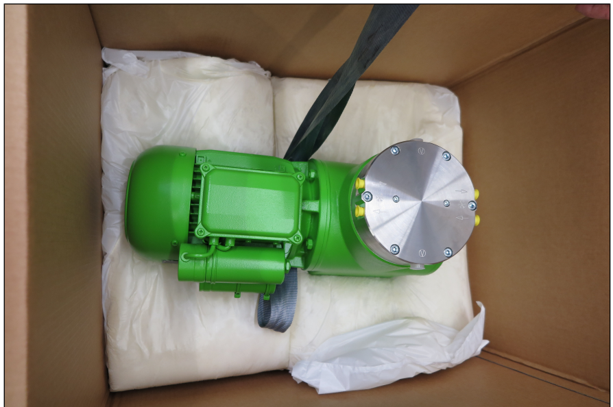
Fig.4 Position of carrying strap (example)
