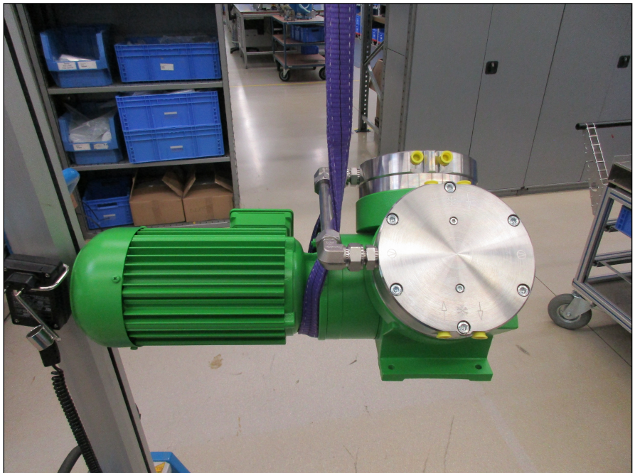
Fig.7 Fastening the carrying strap (pump shown as an example)
