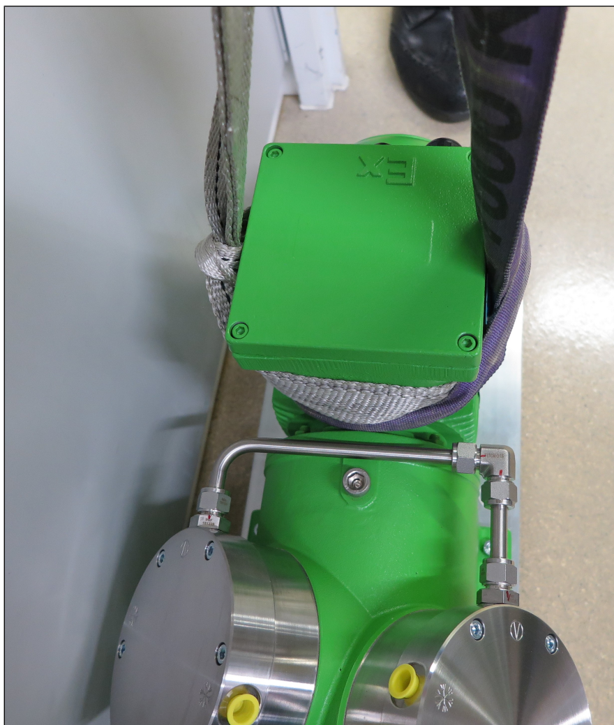
Fig.20 Lifting motor (depicted pump as an example)
