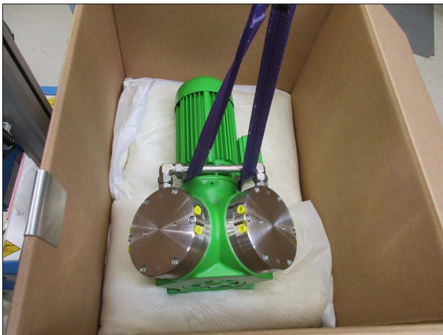
Fig.6 Position of carrying strap (example)
