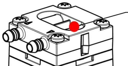
Measurement position for highest temperature, pressure side
