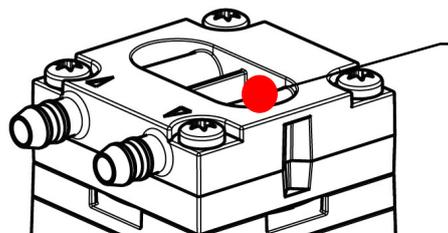
Measurement position for highest temperature, pressure side
