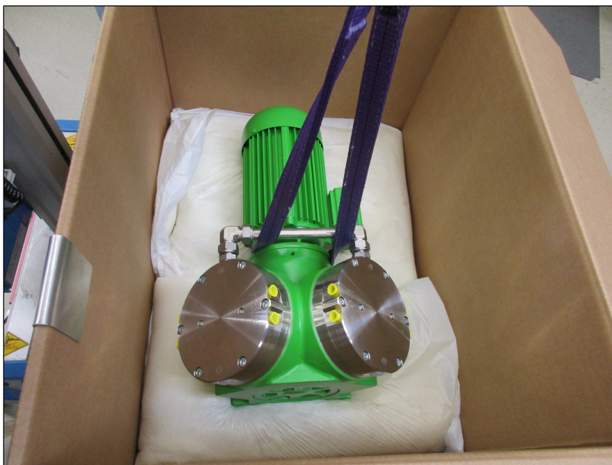
Fig.5 Position of carrying strap (example)
