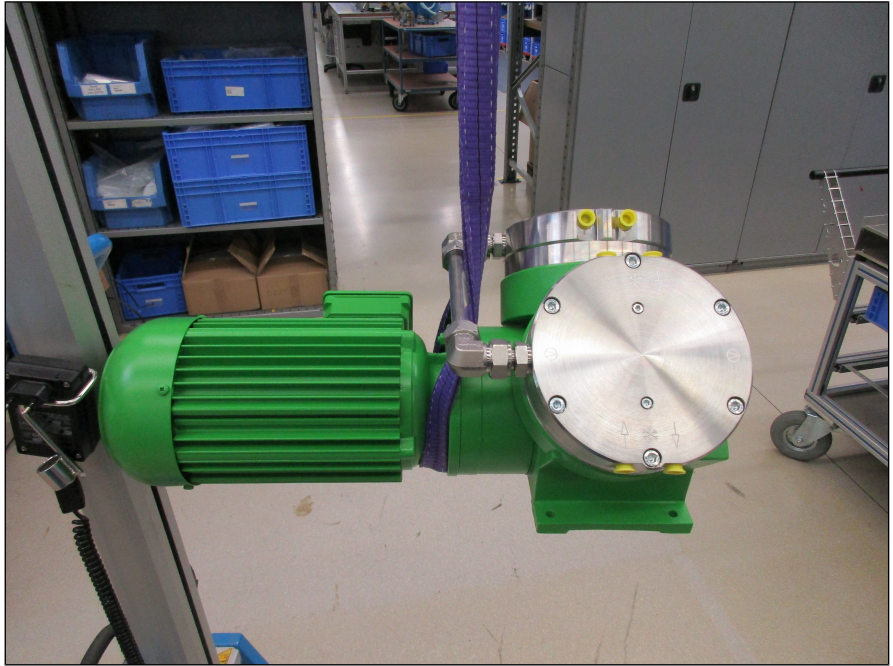
Fig.6 Fastening the carrying strap (pump shown as an example)
