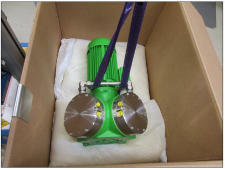
Fig.6 Position of carrying strap (example)1. Pull the carrying strap under the pump (see Fig. 6).
