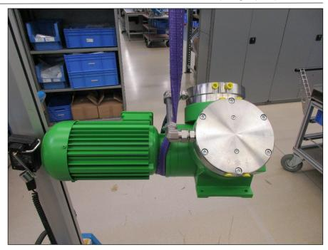
Fig.5 Fastening the carrying strap (pump shown as an example)
