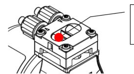
Measurement position for highest temperature, pressure side
