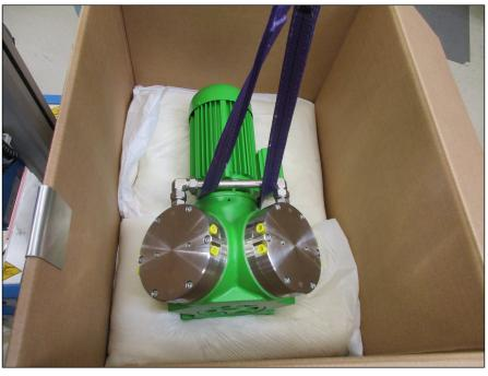
Fig.5 Position of carrying strap (example)
