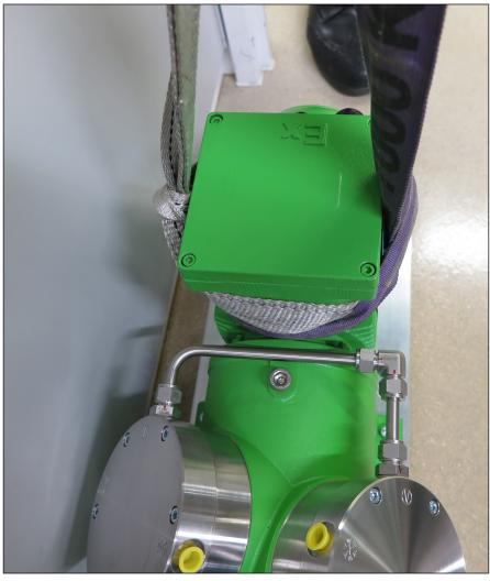
Fig.18 Lifting motor (depicted pump as an example)
