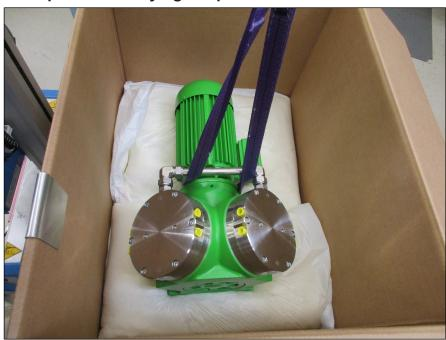
Fig.5 Position of carrying strap (example)
