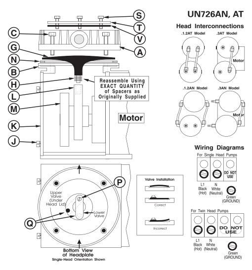
Ensure that the compression rings (ferrules) are correctly positioned under the union nuts before tightening the interconnection fittings.
